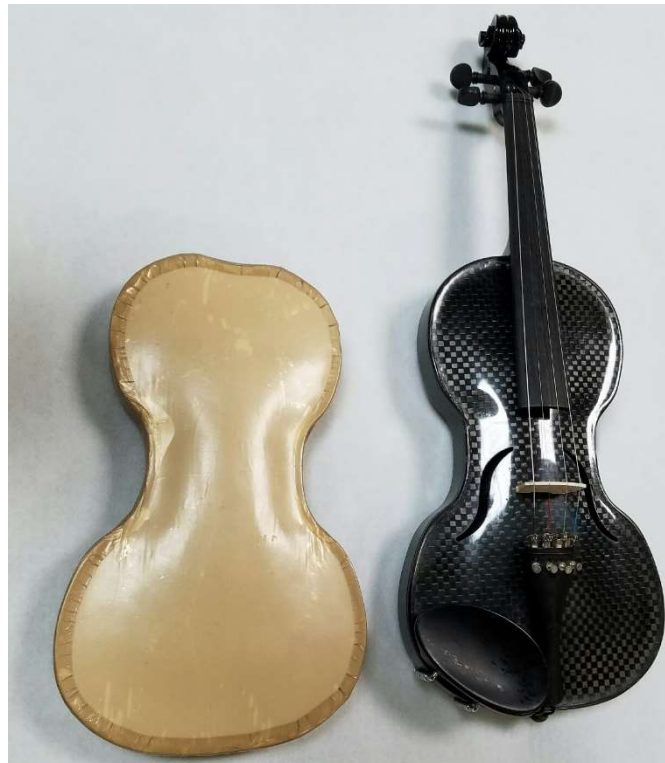
Figure 1. ClaveCore mandrel and composite violin fabricated from 350°F prepreg.
