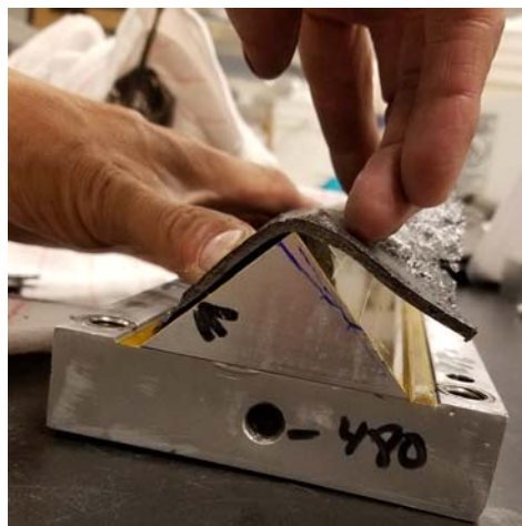
Figure 2. ClaveCore Film HT application demonstration. Film easily conforms around 90° corner.
