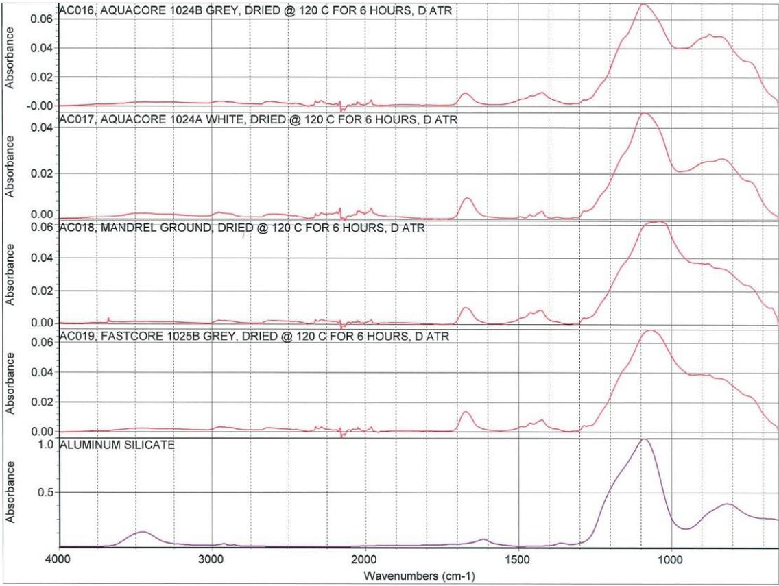
**Figure 3. FTIR analysis of water soluble mandrel materials.**
