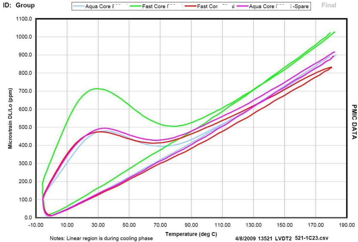
**Figure 1. Expansion during thermal cycling.**
