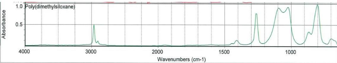
**Figure 4. FTIR spectra of silicone reference.**
