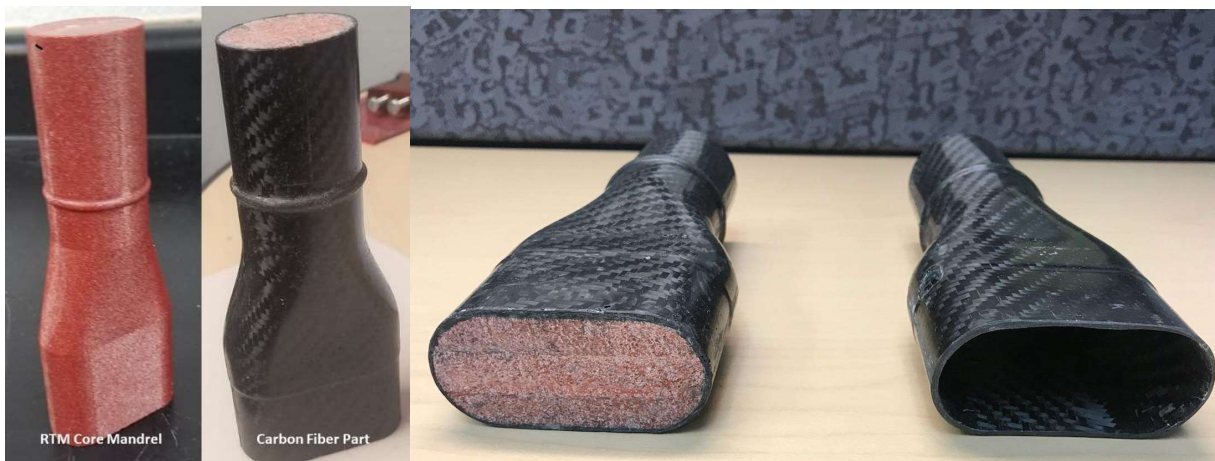
Figure 1. RTM Core mandrel and composite nozzle.
